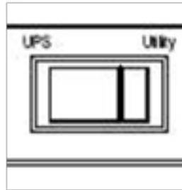
**XBDM Bypass Switch – UPS Position**
