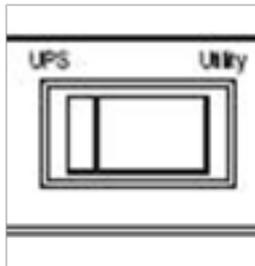
**Figure 23 – XBDM Bypass Switch - UTILITY**
